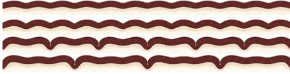
Figure 17 Emerging instability patterns of primary and secondary bifurcations. Moderate growth beyond the first instability point creates a symmetric, sinusoidal wrinkling pattern. Further growth triggers symmetry breaking into a nonsymmetric pattern with sharper valleys and smoother ridges. Continuing growth beyond a second instability point initiates period doubling or period tripling with increasing and decreasing amplitudes (Budday, Kuhl, & Hutchinson, 2015).
